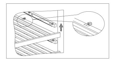
Put the shelf gap(left and right) under the square plastic block, uptilt the shelf,then pull the shelf from the Wine Cooler.
